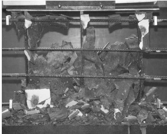
a) specimen with rebars only (applied tensile strain is 1.5 ‰)
