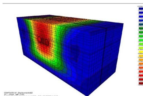
Figure 3. 3D FEM mesh for the portion of two parallel tunnels (Postolskaya et al., 2001)
