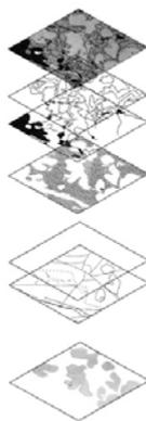
Figure 1. Layers represented in GIS for the near-surface portion of the rock/soil mass at a potential site (Postolskaya et al., 2001); <http://www.gis.com/>
